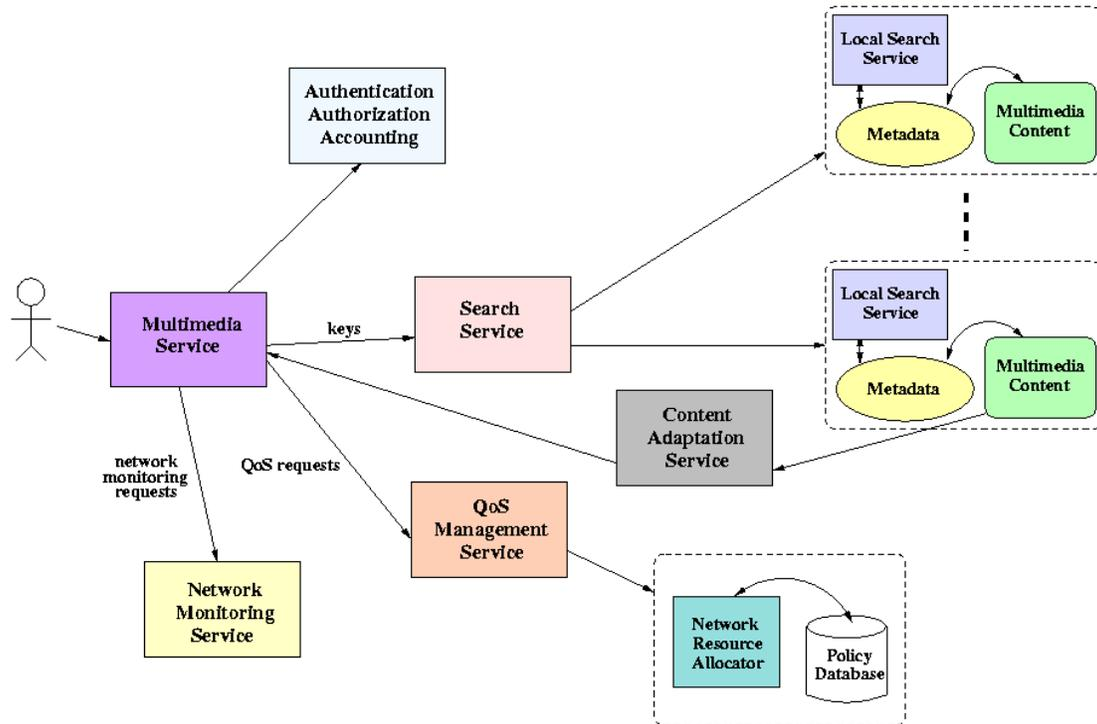
Figure 1: High-level organization of the service-oriented multimedia distribution architecture.
