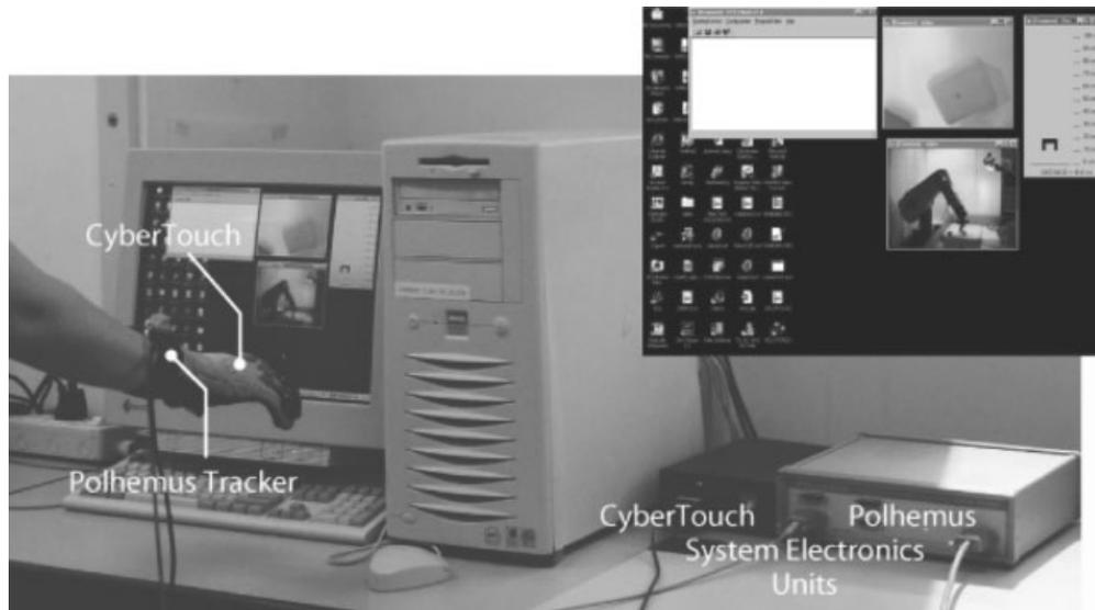
**Figure 13.** An example of the Client Setup and a snapshot of the output with windows displaying sensory information received from the remote site.
