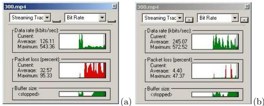
Figure 1: *Quicktime network statistics for best delivery (a) and QoS enabled (b) streaming sessions for a 802.11b wireless client.*
