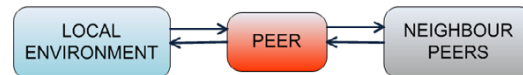
Figure 2: Interactions between a peer, its local environment and its neighbors in a traditional P2P architecture.
