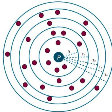
Fig. 1: In the DGT-based proactive localization protocol, each node's concentric data structures (GeoBuckets) are centered on the node itself.
